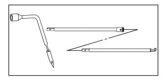
Assemble the wheel wrench (D), the jack handle extensions (A) and the jack handle (C) as shown.
